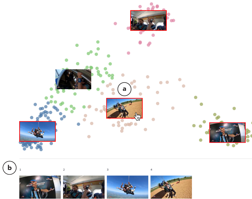
Figure 7: VideoMap’s Project Panel can be extended to create summary videos. We automatically create “semantic districts” that approximately represent the main activities of a video using k -means clustering under the semantic lens. The editor can select several landmarks to specify the activities to include in the summary video. Selections are highlighted with red borders (a) and displayed as a storyboard (b).
